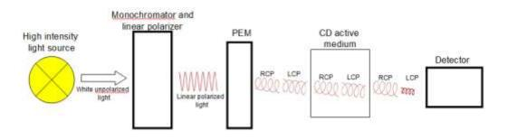
FIG 5:- CD SPECTROSCOPY METHOD OF WORKING
