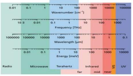
Figure 2 The electromagnetic spectrum showing terahertznradiation in relation to adjacent spectral regimes.<sup>[9]</sup>
