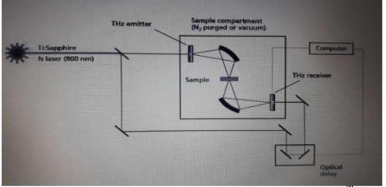
FIG 7:- TERAHERTZ PULSED APECTROSCOPY METHOD OF WORKING<sup>[9]</sup>
