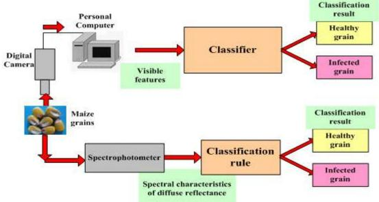
FIG 4:- INFRARAD SPECTROSCOPY METHOD OF WORKING
